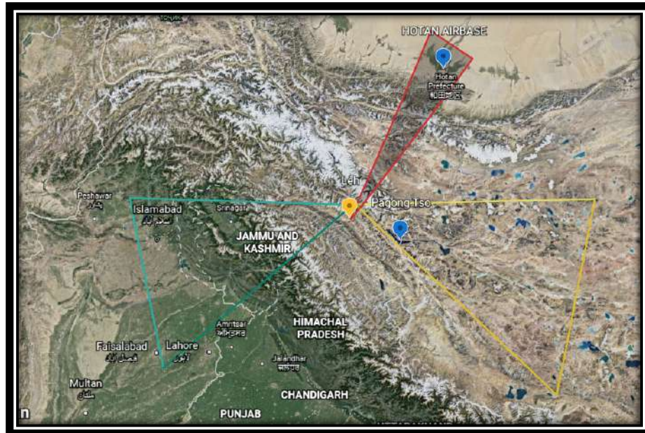
Figure 5: Ground Coverage Area of a HALE at 65,000 feet in Indian Context
