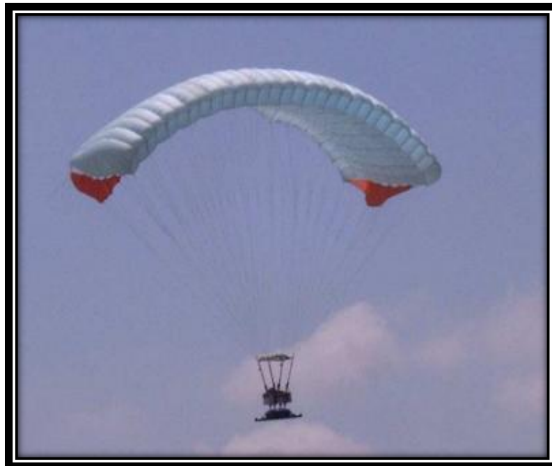
Figure 3: An Aerial Delivery System During Flight
