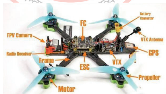
Figure 1: Parts of FPV drone
